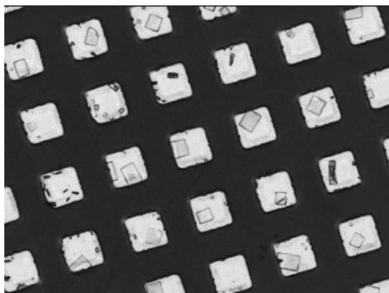
Fig. 5. Regular K_2SO_4 crystals in an array of microvessels with hydrophilized bottoms. They were obtained after dip coating the plate into 10 wt.% aqueous K_2SO_4 solution. Their quality was improved by three cycles of condensation and slow evaporation of the water using a Peltier element to cool the microarray slightly below room temperature. The image was taken with a light microscope. Each microvessel is 50 \mu m wide.
